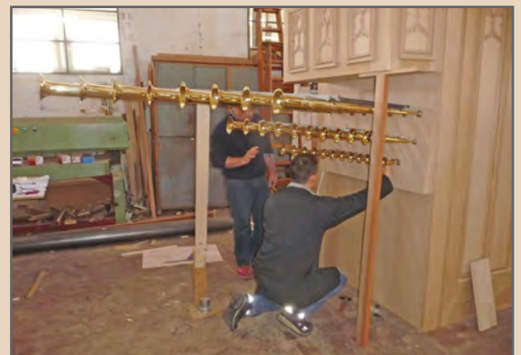
At right, the brass horizontal Pontifical Trumpet resonators, which will face the nave from the West Gallery organ cases.
