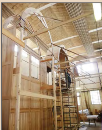
At left is one of the Quire cases, shown during assembly at the Ruffatti factory.
