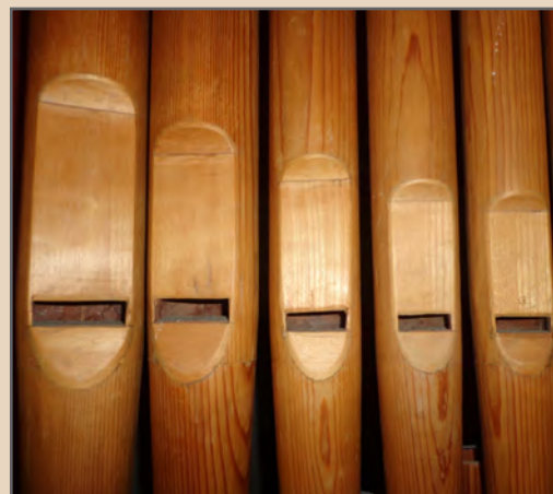
Spruce façade pipes, rounded like metal pipes, with carved-out mouths in the Church of S. Nicolò in Fusine, Italy.
